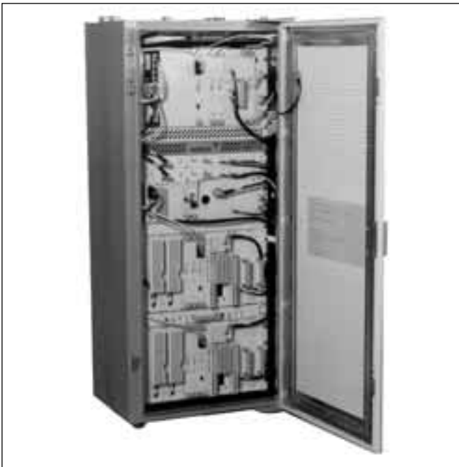
Base station of cellular network
